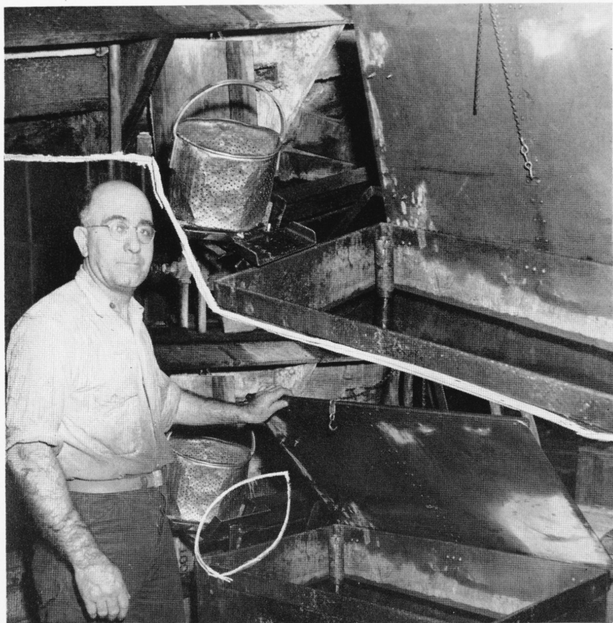
The Cleaning Room originated a novel safety device a short while ago for its tanks of varsol, a flammable cleaning fluid, which must have covers that close automatically in case of fire. Matthew Monzillo poses for the camera.
